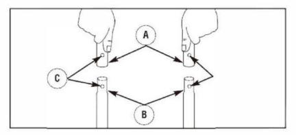
**NOTE:** It may be necessary to move the handle supports from side to side in order to align the handle so it will slide over the handle supports. Hold the location pin in the wheel set backward in horizontal level and press the locating pin into supporting tube until the click is heard, which indicates the pin clutches at the supporting tube.(P1)
