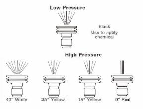
1. Pull back collar on quick-connect and pull current spray tip
