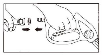
2. Connect spray wand to gun. Tighten securely.
