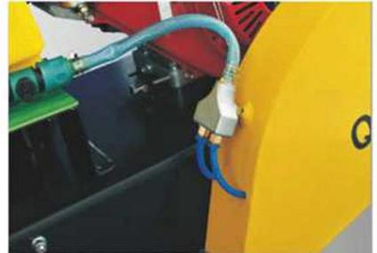
Double water pipe for cooling both sides of blade
