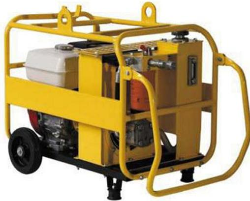
Hydraulic power units, with high efficiency and small size and high reliability and lower noise and light weight, power impacting energy and lower feedback energy, which are greatly used in highway, bridge, expressway, railway, municipality, gas, water, rescue, power, construction etc.
